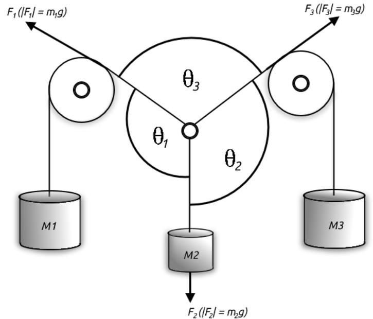
Figure 1.2: Apparatus with vectors ( $\vec{v}$ ) & angles ( $\theta$ )
