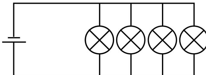
Four bulbs in parallel in our experiment would have the same brightness and would all have  $4.4V$  and  $0.25Amps$ .
