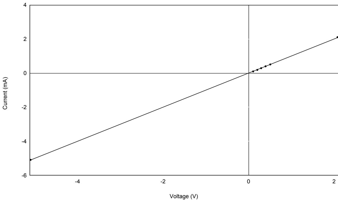
Figure 3.3: Red LED Voltage vs Current
