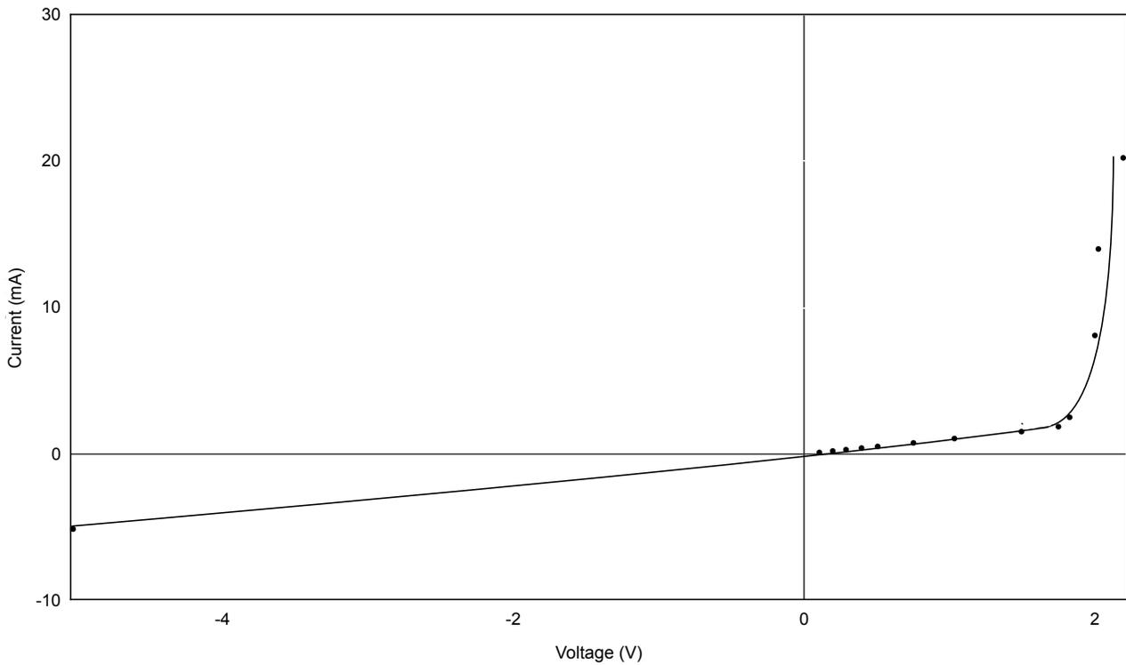
Figure 3.4: Green LED Voltage vs Current
