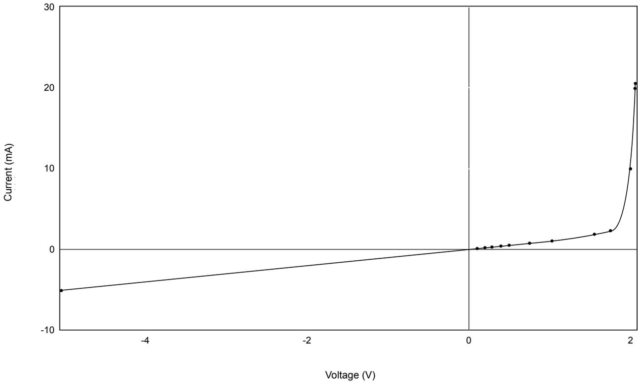
Figure 3.5: Yellow LED Voltage vs Current
