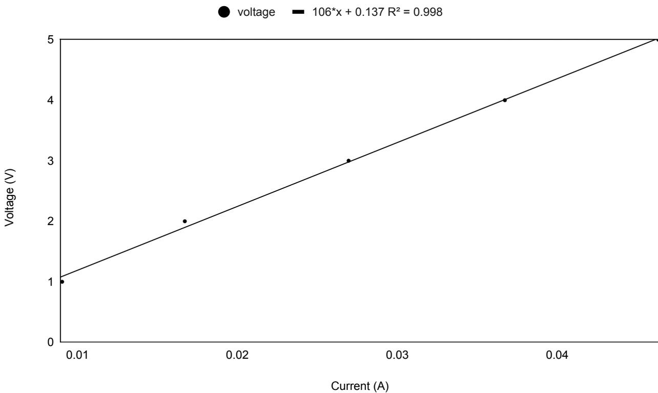
Figure 3.1: Current vs Voltage (100Ω)
